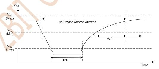
Figure 8.2 Power-Down and Voltage Drop
