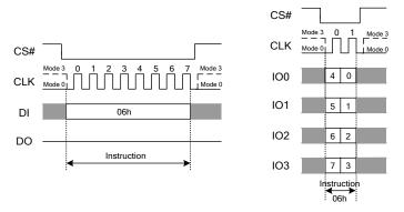
Figure 7.2 Write Enable Instruction(SPI or QPI Mode)
