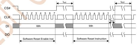
Figure 8.7 Software Reset Input Timing
