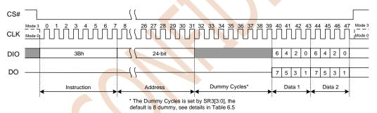
Figure 7.15 Fast Read Dual Output Instruction Sequence Diagram
