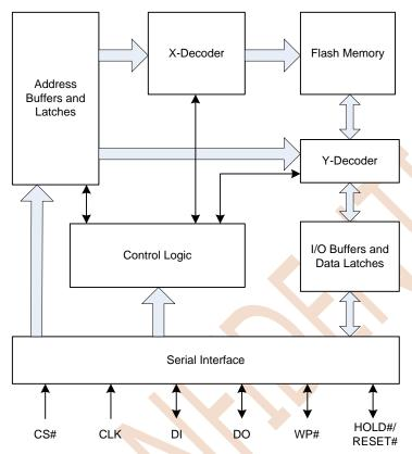
Figure 2.1 Block Diagram
